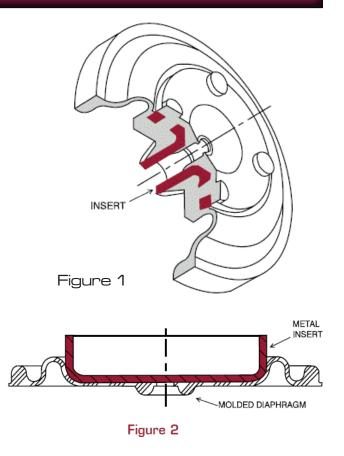
that is compatible with these harsh environments without limiting the life and responsiveness of the diaphragm. For additional strength, fabric reinforcement may be added to the PTFE/Elastomer composite. Bonded inserts of stainless steel, brass, plastic, and cold-rolled steel are often incorporated into these diaphragms to reduce process/ assembly steps and add value.
