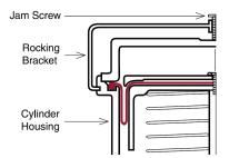
Provides quick assembly and disassembly. The pivoted rocking bracket is attached to the housing flange and the central jam screw secures the bonnet against the mating flange.
