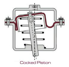
diaphragms do not require lubrication they may be coated with a molybdenum disulfide prior to installation to aid in the reduction of abrasive wear. The piston may also be coated with PTFE to reduce friction when the diaphragm shifts against it, or with an elastomer coating which will prevent the diaphragm from shifting resulting in the elimination of abrasion.
