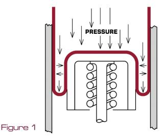
The sum of the vertical components of the unit pressures acting on this semicircular segment add up to the total pressure force (F) and is equal to the normal pressure on the projection of this segment.
