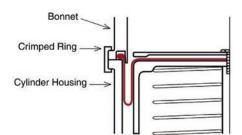
Used in high volume, low cost applications, this method eliminates typical flange construction and flange bolts.
