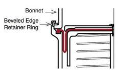
Eliminates the need for flange bolts as a beveled edge ring is snapped into a groove in the extension of the cylinder housing flange. This loads the bonnet assembly onto the mating bead, generally producing low clamping forces.
