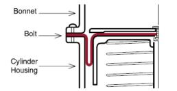
Most common flange retention method. Bolt holes should be at least 15% larger than the bolt. Allow sufficient number of bolt holes to eliminate bowing or distortion of flange, providing a tight seal and preventing the diaphragm flange from pulling out between the bolts.
