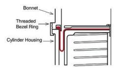
This common method provides minimum clearance of the housing outside diameter. Male threads are machined on the cast bonnet to utilize drawn sheet metal cylinder housings, reducing costs.
