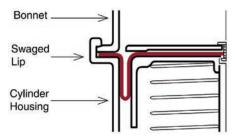
Lending itself to high volume/low cost, the swaged lip resembles the crimp ring in design except that the lip is an integral part of the cylinder or bonnet. Lip should be flexible and thin to insure proper flange retention
