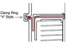
"V" style clamp rings can be disassembled quickly by removing a clamp lever. A retainer plate is removed by turning it 90 degrees where two"wings" and a retaining screw drop into a keyhole.
