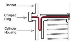
This method lends itself to high volume and low cost manufacture. It utilizes a separate metal crimp ring and is assembled to unit with special crimping tools. These crimp rings are made of thin, ductile materials so that the force required to form the lip will not over-compress the diaphragm flange area.
