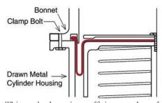
This method requires sufficient number of circumferential clamp bolts so distortion does not occur between flange bolts. It is advisable to make provisions for the bead groove in the cast or molded bonnet.
