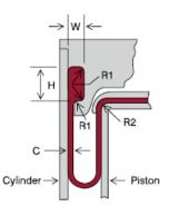
same height. Because the clamping and sealing of this style diaphragm is against the inside wall of the cylinder, the stroke is restricted to the lower half of the diaphragm.
